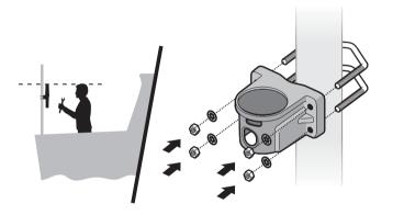
Figure 3 Installing the Identifier bracket
